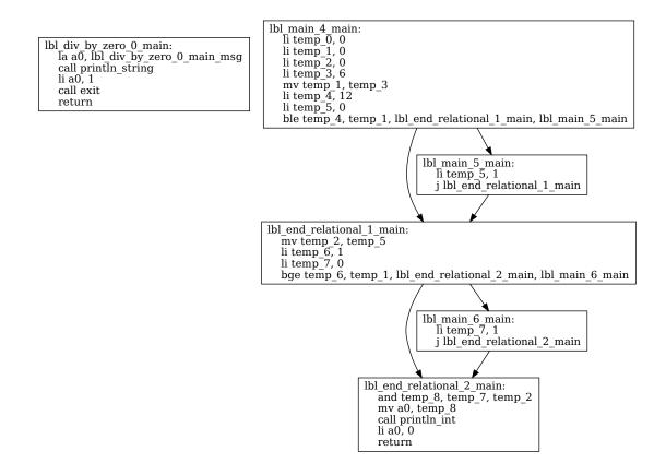
The isolated block in this example corresponds to code related to division by zero. This particular block is added independently from code generation.
